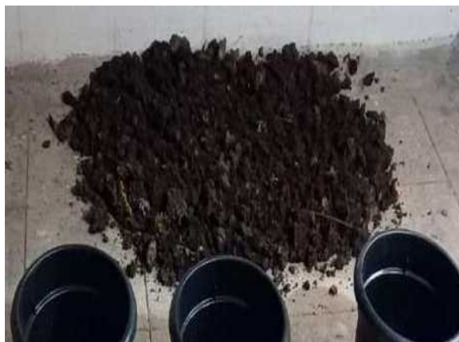
Fig 2. Shade Drying of Sludge
