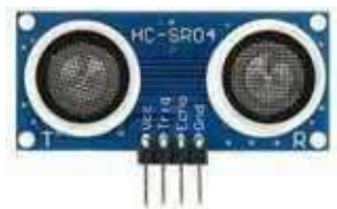
Fig 14. Ultrasonic distance measuring sensor
